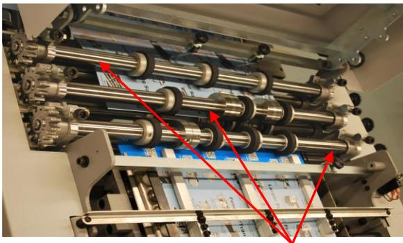
Each BAUM 20 VFM section has three sets of removable cartridge slitter shaft assemblies that use the same tooling as the BAUM 20 folders.
