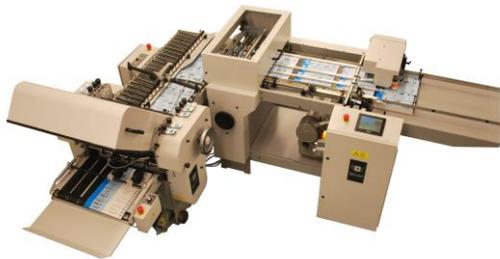
The BAUM 20VFM-1P 1<sup>st</sup> station module with pile feeder register, and scoring unit can be used with a BAUM CF20 Folder allowing you to do scoring, slitting, perforating and folding heavy weight stock all in one pass. The CF20 can handle heavier weight stocks due to its large diameter fold rolls and gear plate drive for the fold rolls.
