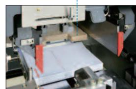
The height of each knife and the angle of the fore-edge knife can be adjusted through the color touch screen during operation. Trimmings are blown away from the knife by strong air nozzles mounted on the knife holders.
