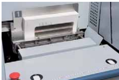
Automated Point Carriage Clamp Width
